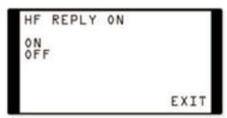
The first line of the display indicates whether Handsfree Reply is on or off.
